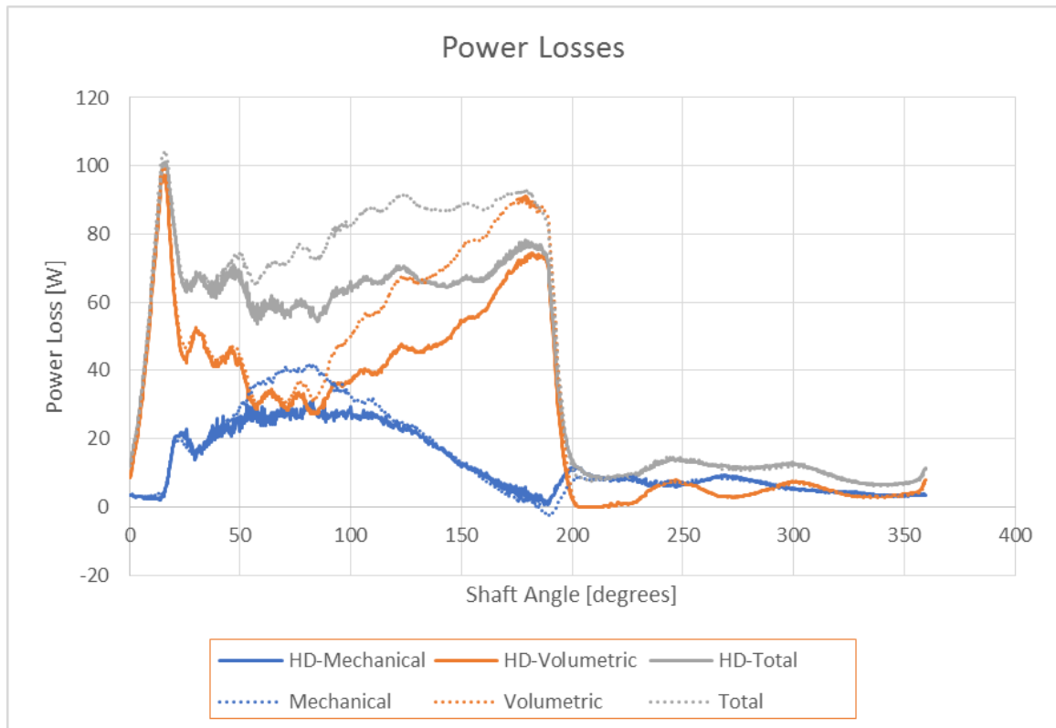
Figure 7.9. Simulated power losses for HD piston cylinder model and standard definition model.
